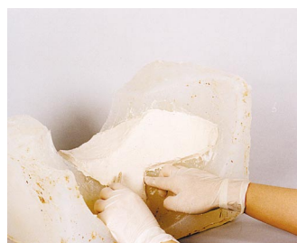
(c) 복원제를 형틀에 눌러서 결실부 제작 The lost part is manufactured while restoration material is pressed to the mold
