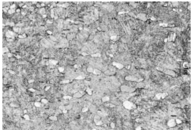
Photo 6-2. Microstructure of bronze bowl II( \times 100 ).
