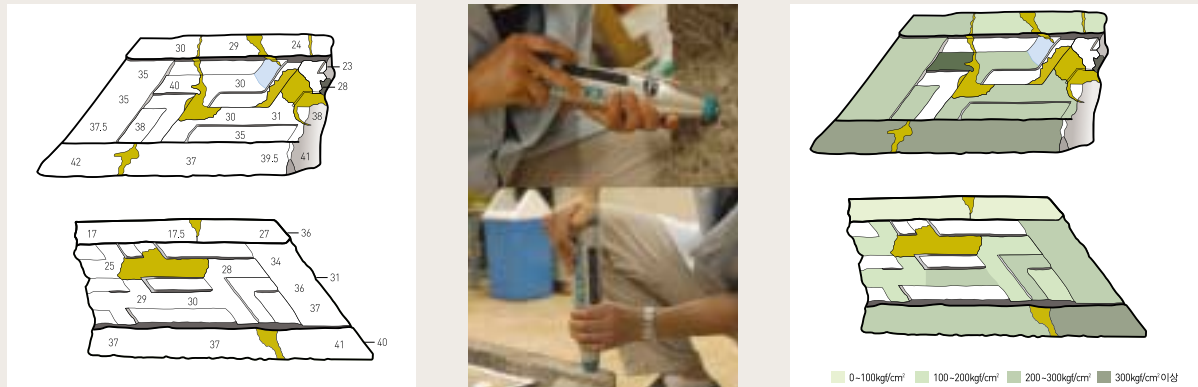
Photo 4. Position of measuring Schmidt Hammer and distribution chart of estimated strength
