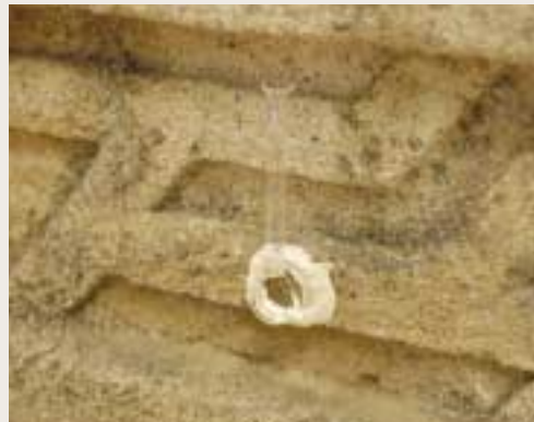
Photo 5. Karsten tube measurement
